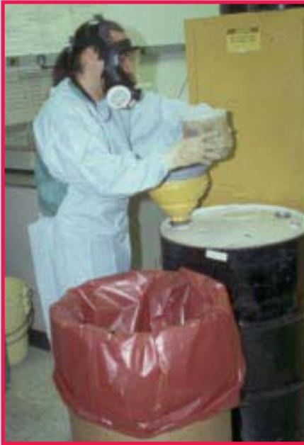
Personal protective equipment required when working with formaldehyde in a poorly ventilated area.
