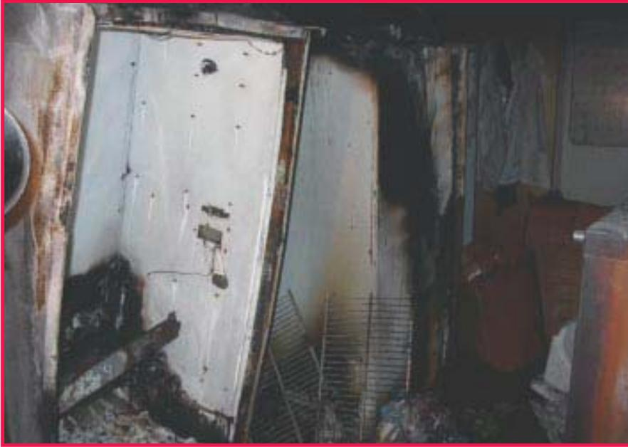
This photo depicts the aftermath of what happens when approximately 50 ml of isopentane is placed in a loosely capped 1-L bottle and the bottle is placed in a freezer that is not explosion-proof. Eventually the freezer thermostat will kick on when the isopentane vapors contained in the freezer are sufficient to support ignition. It's the same basic thing that happens to gasoline vapors in a car engine cylinder ignited by the spark plug. Ignition: Blast Off.
