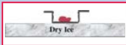
Fig. 2. A solid block of dry ice may be used to freeze tiny samples in molds containing OCT in order to obtain a totally flat block face.
