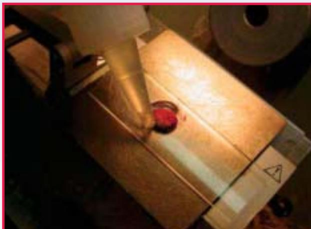
Fig. 5A. Tissue is placed onto the cryostat freeze bar and lightly coated with OCT while a chuck is prepared. In this photo, the knife holder was used to facilitate photography only, and is not intended to be used in this technique.
