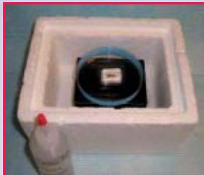
Fig. 4. Plastic Petri dish (blue) is supported by a platform to prevent tipping into the LiqN<sub>2</sub> inside a styrofoam box.
