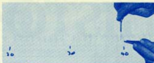
FIGURE 3: Sections numbered in desired intervals with a felt-tip pen and cut from the ribbon with light pressure.
