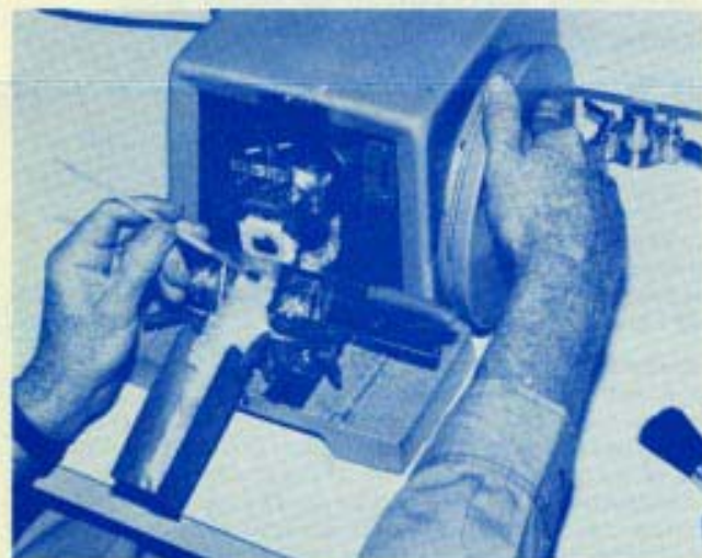
FIGURE 2: Device inserted under the clamped knife mount and sectioning commenced.
