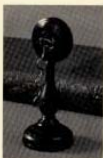
Simple microscope, spring object holder replica, early 19th century. Basically a magnifying glass, this lignum vitae microscope demonstrates the simplest form of controlling the specimen/lens distance.
