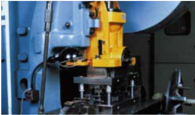
Blade Punching: Quality-inspected materials are punched into final blade shape.
