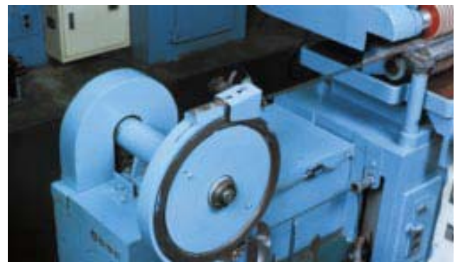
Edge Grinding: Precision grinding, within microns of tolerance, create exact blade angles and triple-honed shape — all performed in line on grinding machines manufactured by Feather.
