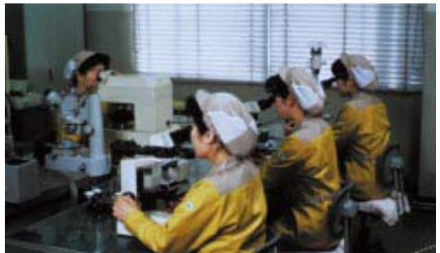
Intermediate Inspection: All disposable blades are inspected throughout the entire manufacturing process.
