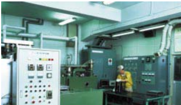
Platinum Coating: Platinum and chrome coatings are added to reinforce blade edge strength and durability.
