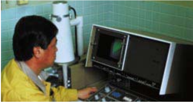
QC Testing: All disposable blades are fully inspected to ensure consistent quality. The microtome sectioning test is performed lot by lot.
