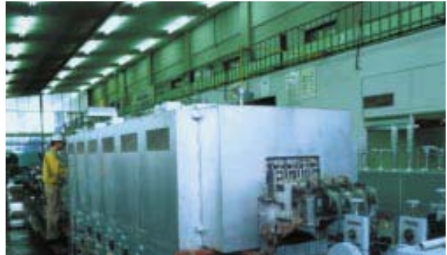
Heat Treatment Processing: Using a special high-heat treatment with "flash cooling" tempering assures the proper combination of hardening and flexibility in every Accu-Edge blade.
