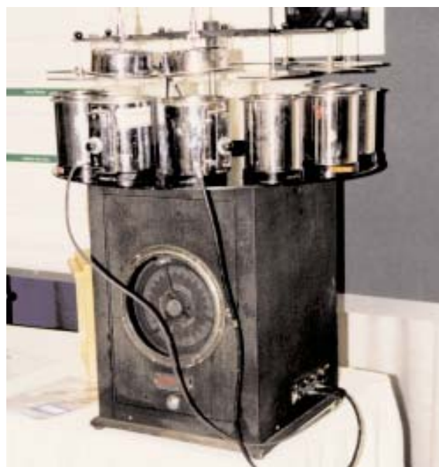
Automation entered the histology laboratory with the introduction of the Autotechnicon® in 1939.
