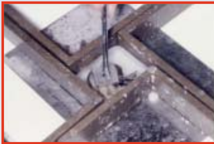
Fig. 3. Embedding oversized specimen using lead Ls.
